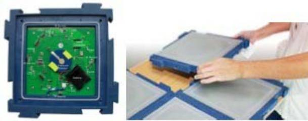
Figure A.1: Left: The interior of the modular interactive tiles. Right: Assembling of a tile play field. Intervention
